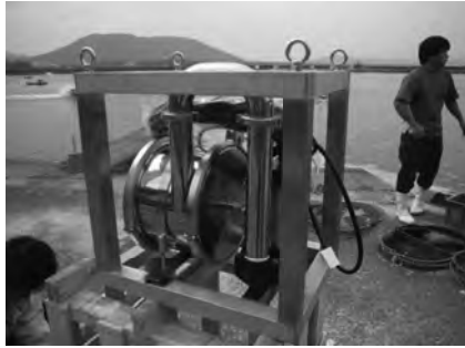
Photo 2.3 Microbubble generator \phi 300 mm for shrimp ponds.
