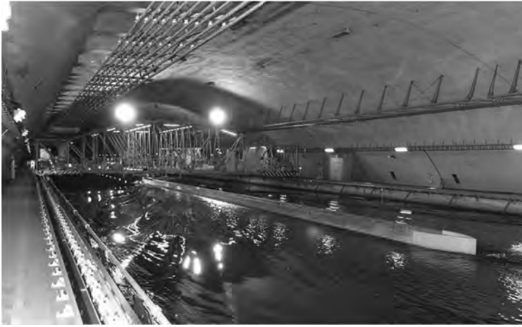
Figure 10.4 An air bubble experiment using a flat plate of 50 m length and 1 m width [14,15].
