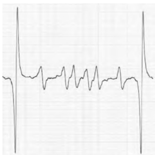
Figure 4.2 ESR spectra of microbubbles in distilled water, using DMPO as a spin-trapping reagent for oxygen microbubbles.
