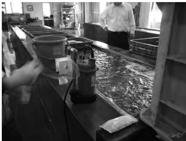
Photo 2.8 Medium-sized bubble generation device status ( \phi 75 ) set.
