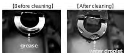
Figure 5.7 Photographs of a test piece stained with hydrophobic grease (left side) before and (right side) after 10 s microbubble cleaning.
