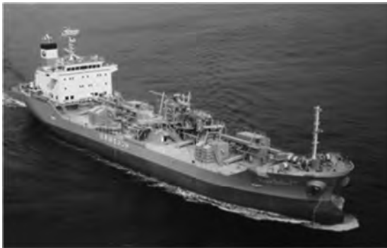
Figure 10.7 The cement carrier “PACIFIC SEAGULL” used in the full-scale air bubble experiments [21] ( L_{pp} = 120 m, width = 21.4 m, gross tonnage = 7809 tons, draft at full load = 7.215 m).
