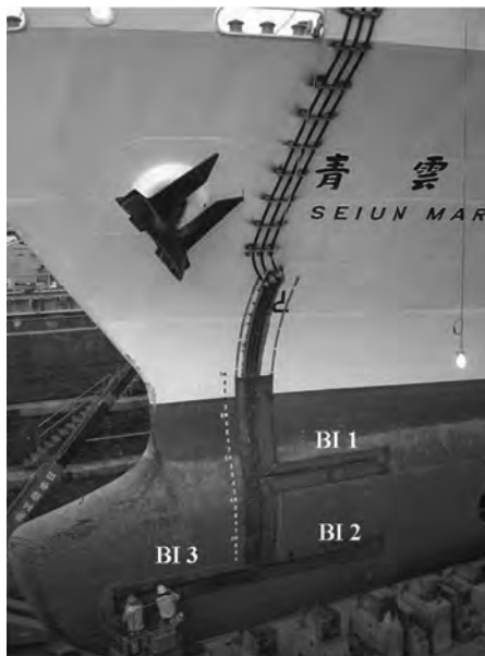
Figure 10.6 Bubble injectors (BI-1 through BI-3) attached near the bow of SIRUN-MARU [18].
